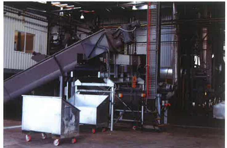
Primary metal detector which reverses when metal is found and deposits it in the bin for removal by hand. Picks up items as small as a foil wrapper.
